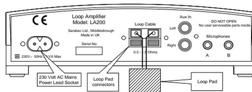
Connect one wire of the lead to the right hand terminal (RED) and the other wire in the lead to the left hand terminal (BLACK).
