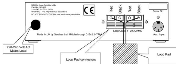
Connect one wire of the lead to the left hand terminal (RED) and the other wire in the lead to the right hand terminal (BLACK). No wires should be placed in the inner pair of terminals.
