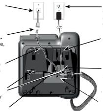
Plug the large end of the telephone base power adapter into a power outlet.
