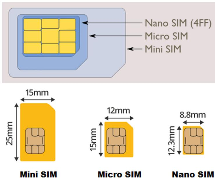
**Mini SIM (2FF) [Standard SIM]** – A mini SIM card is also called the standard SIM card or regular SIM card size and it was used by millions of mobile phones until now because today all the modern day Smartphones generally comes with micro SIM or nano SIM card slot. The dimensions of mini-SIM are 25mm x 15mm x 0.76mm.
